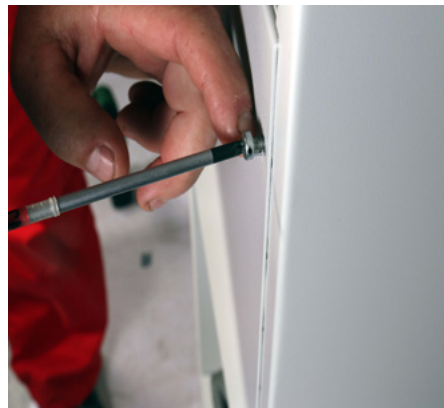
The tap should penetrate the hole, and the screw fastened.
