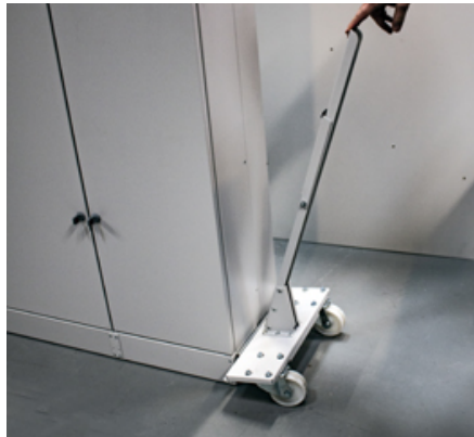
Use transport device to lift panel from the floor
