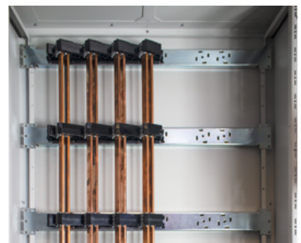
Example of vertical fitting, here stop pads should be mounted at both ends. Busbar: 4821-00X0
