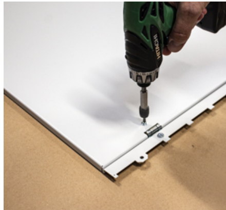
Hinge must be mounted in the front with brackets
