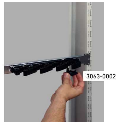
Busbar holder should be clicked on either horizontally or vertically, and stop pads mounted at the bottom of the column.
